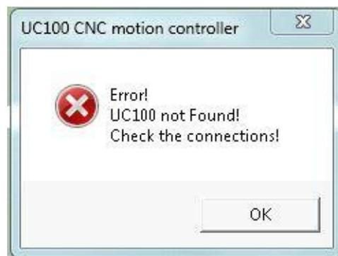
The following popup screen appears if Mach3 losing the connection with the UC100 meanwhile it is operating. This event may happen if the USB cable is broken or if the cable connector was accidentally slipping out from the UC100 or from the PC. The workaround is checking the USB cable connections and plug it back and restart Mach3.
