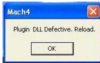
then the .NET framework was not installed on the computer. The .NET framework 2.0 is the prerequisite for running the UC100 controller plugin. The framework can be downloaded from Microsoft's website. The .Net framework 2.0 is part of Windows7 and therefore it is not required to install it on Windows 7 operating systems. It is only required to install it on Windows XP as it not containing this tool by default, it must be installed separately, by the user on the Windows XP operating system.
